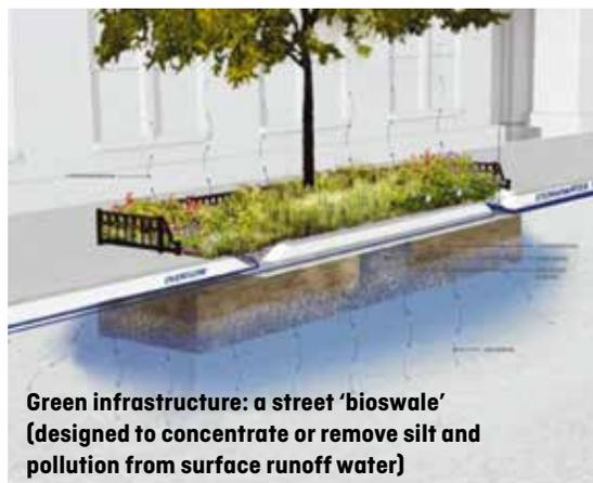
**Green infrastructure: a street 'bioswale' (designed to concentrate or remove silt and pollution from surface runoff water)**
